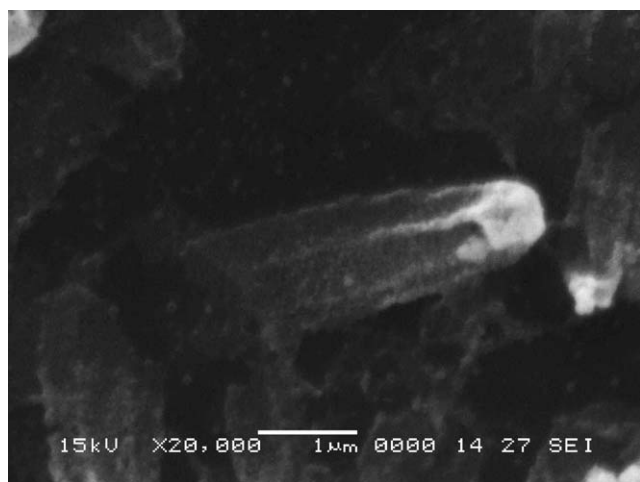
Fig. 2. SEM image of a single hollowed hexagonal gold tube on membrane.
